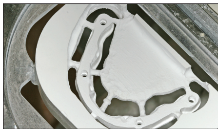
Fig. B The framework is milled from the zirconia block.
