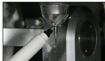
Fig. F For the "drop the pin" milling technique, the milling bur is dropped approximately 0.75mm...
